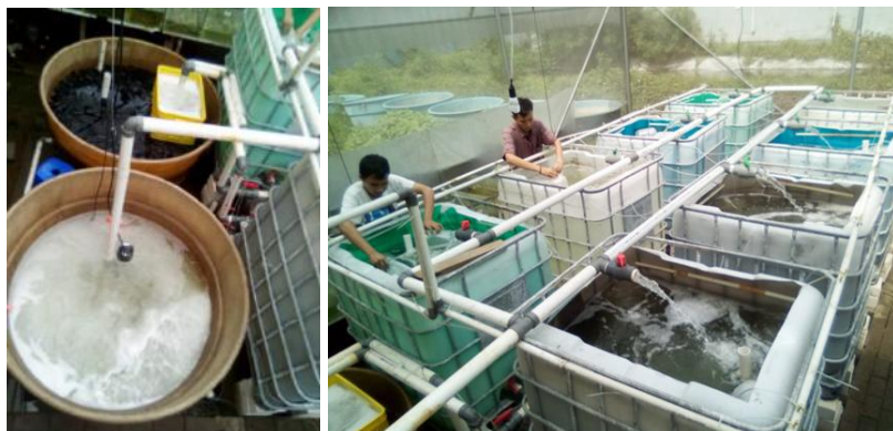
Fig 41: Application of a recirculating aquaculture system (RAS) for Litopenaeus vannamei culture in Indonesia. The system has a total water capacity of 8.5 m 3 and is equipped with a physical filter, bioblock biofilter and microbubble technology for aeration and organic particulate removal.
